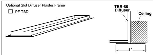
The PF-TBD slot diffuser mounting frame can be used in sheetrock or plaster ceiling. The frame is mounted in the ceiling by others. The Model TBR-80 is mounted on the inside lip of the frame. Plaster frame is 1 ½" high.
